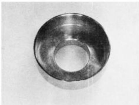
3650523 Use to hold 1st Lens Group in Tool No. 3650533 and centering microscope.
