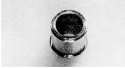
3650526 Use to hold diaphragm housing when centering 4th Lens element and to hold lens barrel when centering 2nd Lens Group in lens barrel.
