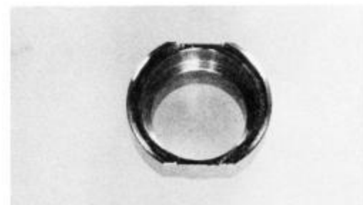
3650525 Use to hold 3rd Lens Group frame when centering in frame. Use together with 3650533.
