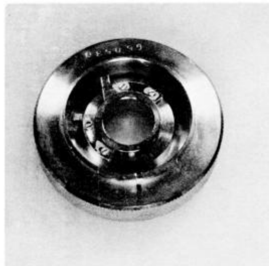
3650530 Use to position stop plates – Canon Mount.
