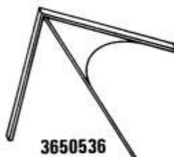
3650536 Use to place scribe lines on Helicoid.
