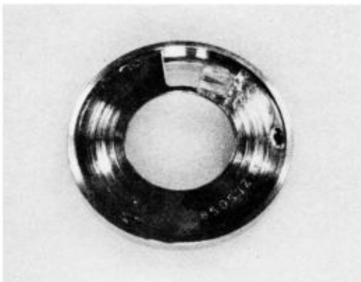
3650532 Use to set position and height of diaphragm coupling arm - Olympus Mount.
