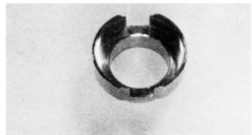
3650524 Use to hold 2nd Lens Group frame when centering 2nd Lens Group in frame.
